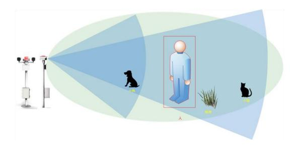
■ The difference between microwave radar and infrared detection sensor
