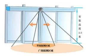
**Opening of the automatic door:** After the detecting personnel approach the gate, the system is notified to open the corresponding motor.
