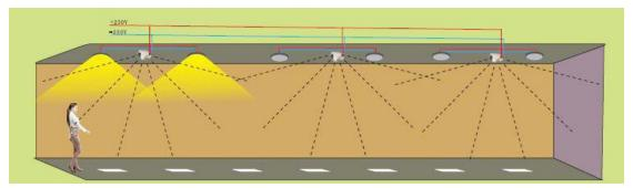
**Intelligent corridor lights:** evenly distribute the sensors according to the length of the corridor. When the person moves, the sensor commands the system to turn on the corresponding light.
