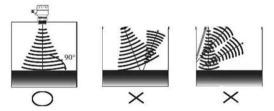
Sound wave incident angle must be at right angles to the horizontal plane
