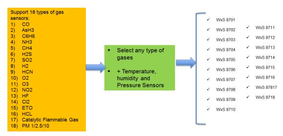
External sensors (outside the enclosure): in addition to internal sensors, listed in the table above, an array of sensors can be externally connected to WxS 8800 via analog or digital input interfaces (collectively called MPI – Multi-Purpose Interface), including:
