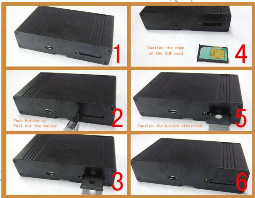
Figure 17: Installation of SIM Card
