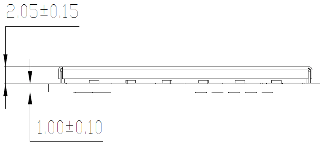
Figure 5: SIM900D side mechanical dimensions (Unit: mm)
