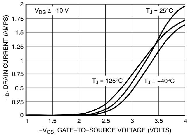
Figure 2. Transfer Characteristics
