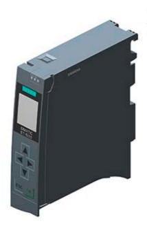
SIMATIC S7-1500, CPU 1513-1 PN, CENTRAL PROCESSING UNIT WITH WORKING MEMORY 300 KB FOR PROGRAM AND 1.5 MB FOR DATA, 1. INTERFACE: PROFINET IRT WITH 2 PORT SWITCH, 40 NS BIT-PERFORMANCE, SIMATIC MEMORY CARD NECESSARY
