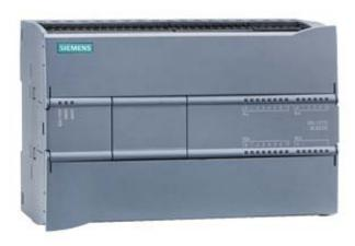
SIMATIC S7-1200, CPU 1217C, COMPACT CPU, DC/DC/DC, 2 PROFINET PORT ONBOARD I/O: 14 DI (10 DI 24VDC / 4 DI 1.5V DC DIFFERENTIAL); 10 DQ (6 DQ 24VDC; 0,5A / 4 DQ 1.5V DC DIFFERENTIAL); 2 AI 0- 10V DC, 2 AQ 0- 20MA; POWER SUPPLY: DC 20.4 - 28.8 V DC, PROGRAM/DATA MEMORY: 125 KB
