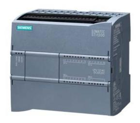
\*\*\* SPARE PART\*\*\* SIMATIC S7-1200, CPU 1214C, COMPACT CPU, DC/DC/DC, ONBOARD I/O: 14 DI 24V DC; 10 DO 24 V DC; 2 AI 0 - 10V DC, POWER SUPPLY: DC 20.4 - 28.8 V DC, PROGRAM/DATA MEMORY: 50 KB
