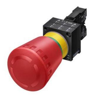
22MM PLASTIC ROUND COMPLETE UNIT COMBINATION: EMERGEN.-STOP MUSHR.PUSHB. 40MM LATCH.W. ROT.-TO-UNLATCH MECH. WITH YELLOW BACKING PLATE SPRING-LOADED TERMINAL, 1NC WITH HOLDER RED INSCRIPTION: NOT-HALT
