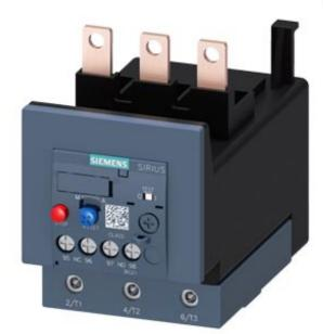
Overload relay 57...75 A for motor protection Size S3, CLASS 10 Contactor mounting Main circuit: Screw Auxiliary circuit: Screw Manual-Automatic-Reset
