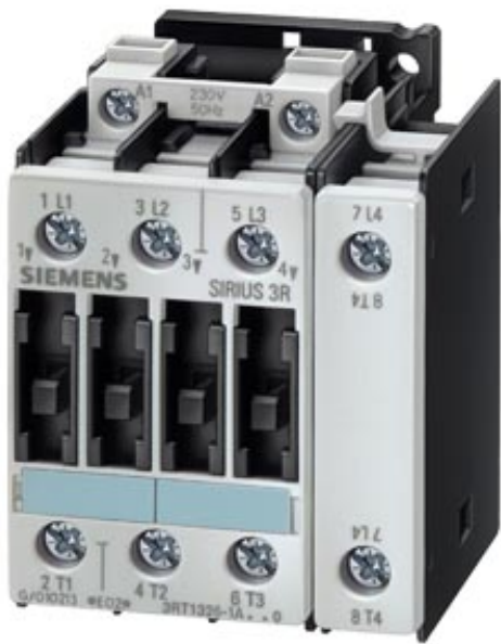
CONTACTOR, AC-1 35A, 22KW/400V, AC 230 V, 50 HZ, 4-POLE, SIZE S0, SCREW CONNECTION
