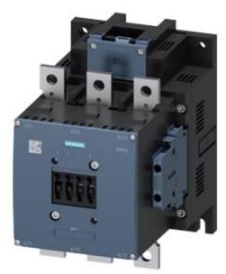
Power contactor, AC-3 300 A, 160 kW / 400 V AC (50-60 Hz) / DC operation 96-127 V UC Auxiliary contacts 2 NO + 2 NC 3-pole, Size S10 Busbar connections Drive: electronic with PLC interface 24 V DC screw terminal
