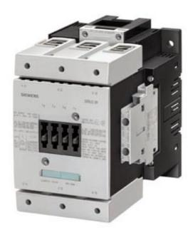
CONTACTOR, 55KW/400V/AC-3, AC(40...60HZ)/DC OPERATION UC 380...420V AUX. CONTACTS 2NO+2NC, 3-POLE, SIZE S6 WITH BOX TERMINALS CONVENTIONAL OPERATING MECHAN. SCREW TERMINAL
