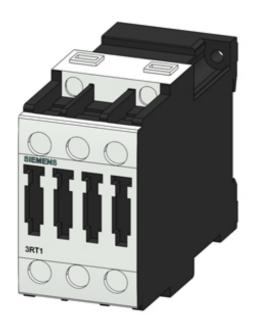
Power contactor, AC-3 9 A, 4 kW / 400 V 24 V DC, 3-pole, Size S0 Screw terminal !!! Phased-out product !!! Successor is SIRIUS 3RT2 Preferred successor type is >>3RT2023-1BB40<<
