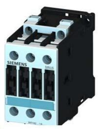
CONTACTOR, AC-3 5,5 KW/400 V, AC 220V 50/60HZ, 3-POLE, SIZE S0, SCREW CONNECTION, MOUNTING POSITION VERTICAL
