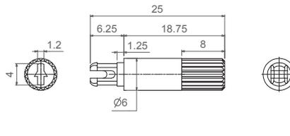
Thumbwheels are available in different colors (color chart in "how to order" section) and with self-extinguishable property according to UL 94 V-0, under request. Thumbwheels can be mounted on the potentiometers at ACP or sold separately. ACP can study special thumbwheel designs.
