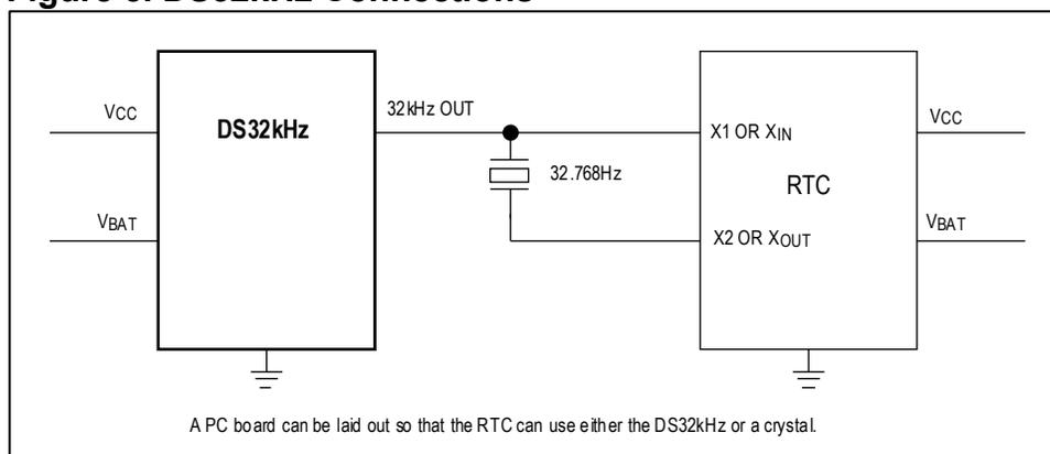
**Figure 6. DS32kHz and RTC Connections**
