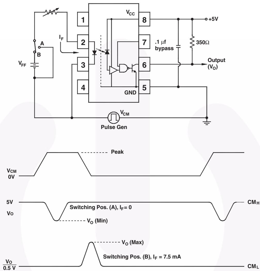
Fig. 14 Test Circuit Common Mode Transient Immunity
