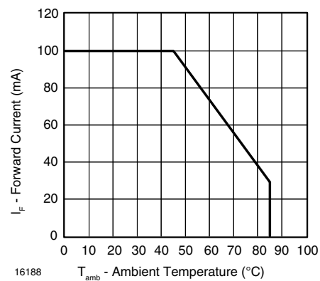
Fig. 2 - Forward Current vs. Ambient Temperature
