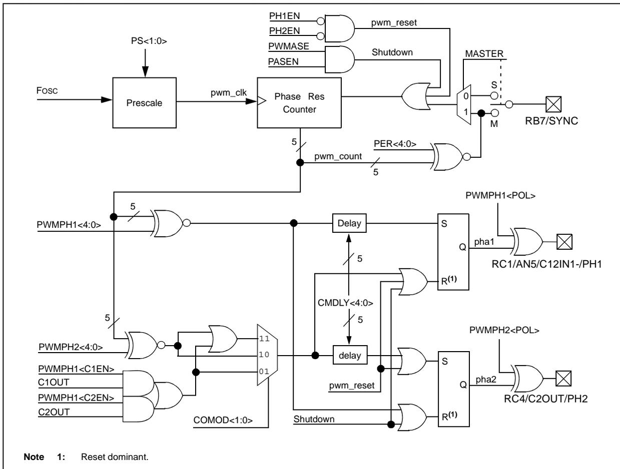
**FIGURE 13-6: COMPLEMENTARY OUTPUT PWM TIMING**
