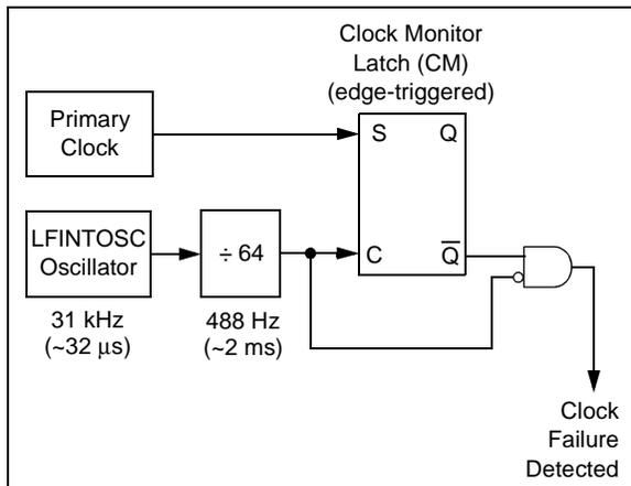
The FSCM sample clock is generated by dividing the LFINTOSC clock by 64. This will allow enough time between FSCM sample clocks for a system clock edge to occur. Figure 3-8 shows the FSCM block diagram.
