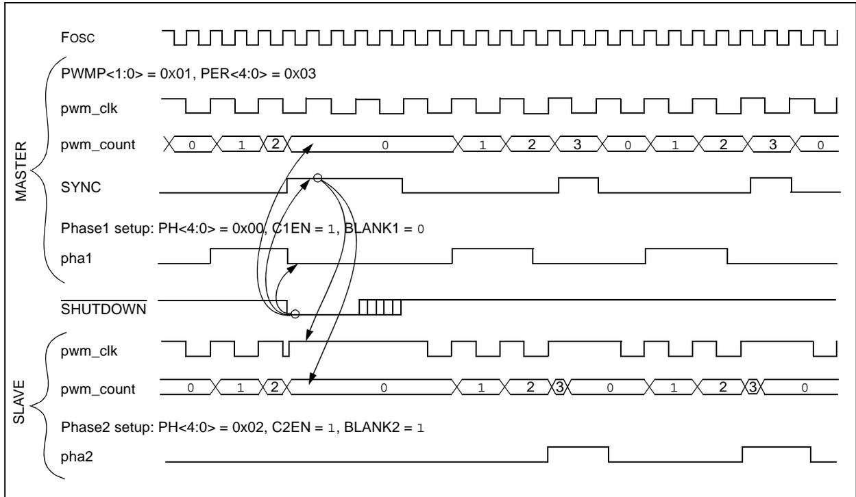
**FIGURE 13-3: TWO-PHASE PWM START-UP TIMING**
