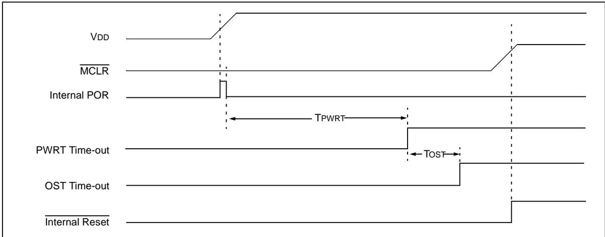
**FIGURE 15-5: TIME-OUT SEQUENCE ON POWER-UP ( $\overline{\text{MCLR}}$  WITH  $V_{DD}$ )**
