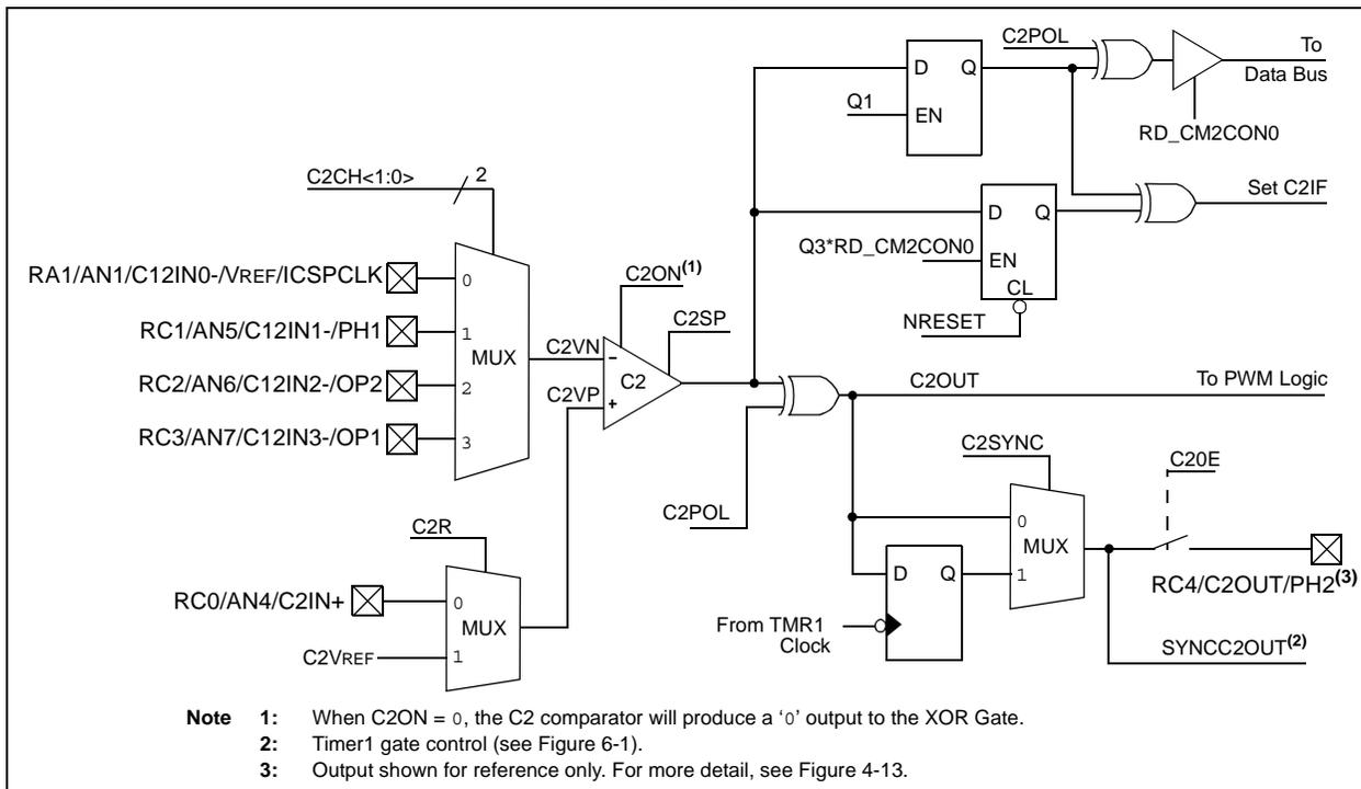
**REGISTER 9-2: CM2CON0 – COMPARATOR C2 CONTROL REGISTER 0 (ADDRESS: 11AH)**
