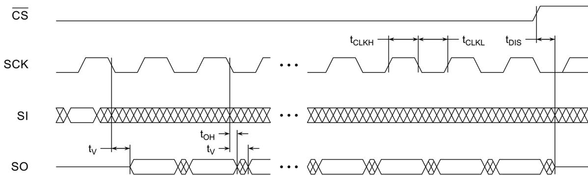
Figure 14-3. WP Timing for Write Status Register Byte 1 Command When SPRL = 1
