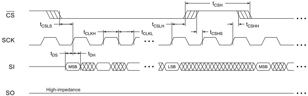
Figure 14-2. Serial Output Timing
