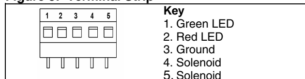
Figure 8: Terminal Strip
