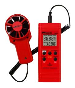
Remote vane with flexible cord helps you place the sensor where you need it, for more accurate measurement results.
