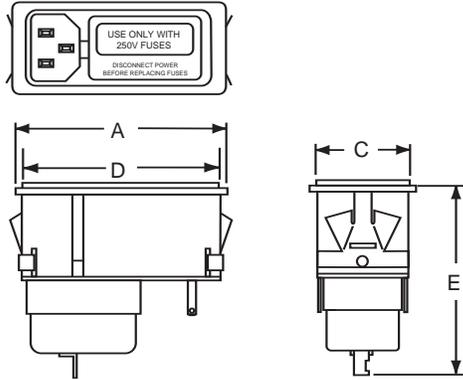
**5EHM1S & 5EFM1S** (IEC Connector, DPST On/Off Switch, Selectable Fuseholder)
