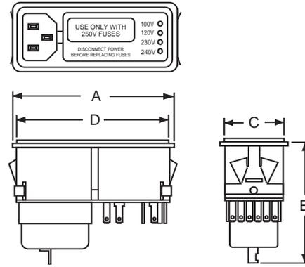
**5EHM4S & 5EFM4S** (IEC Connector, DPST On/Off Switch, Voltage Selector, Selectable Fuseholder)
