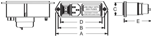
**5EFM1SC** (IEC Connector, DPST On/Off Switch, Selectable Fuseholder)
