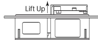
2. Once lifted, the door will pivot on its hinges and expose the fuse holder.
