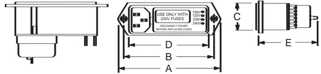
**5EFM4C** (IEC Connector, Voltage Selector, Selectable Fuseholder)
