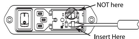
When the fuse holder is installed in the dual fuse position, it will normally release as soon as the door is opened.
