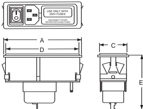
**5EHM4 & 5EFM4** (IEC Connector, DPST On/Off Switch, Selectable Fuseholder)
