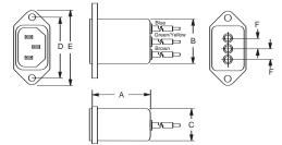
Typical dimensions: Wire leads: 4.0 [*101.6*] Min. 18 AWG Mounting holes: .132 [*3.35*] Dia. (2)
