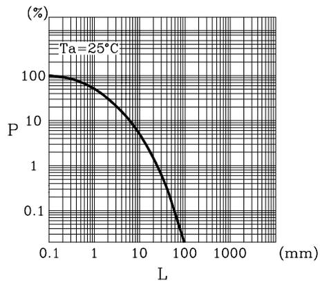
Distance to Detector Test Conditions
