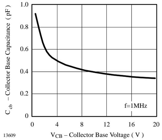
**Figure 3. Collector Base Capacitance vs. Collector Base Voltage**
