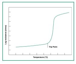
Understanding the differences in performance between the two types of devices will make the best circuit protection choice easier. The most obvious difference is that the PTC is resettable. This is an inherent characteristic in which the PTC resets (returns to low resistance state) after power is removed and the device cools down. There are a number of other operating characteristics that differentiate the two types of products.
