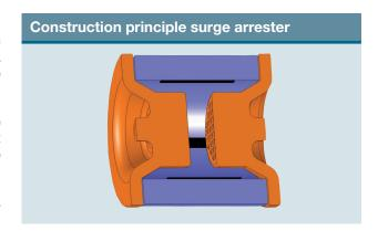
chamber, which is filled with gas and is hermetically sealed, thus secures operation even under harsh environmental conditions such as high air humidity, pollution and strong temperature variations.
