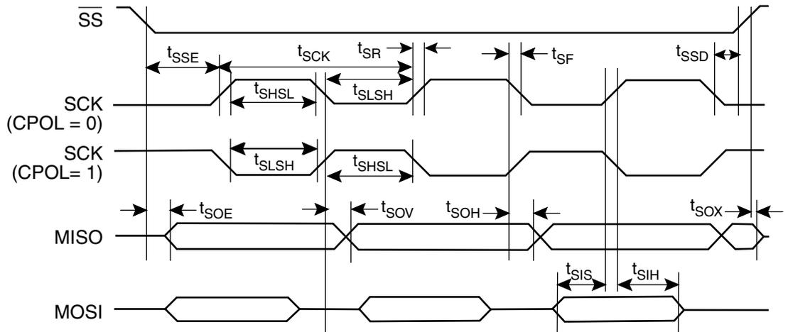
**Figure 15-6. SPI Master Timing (CPHA = 1)**
