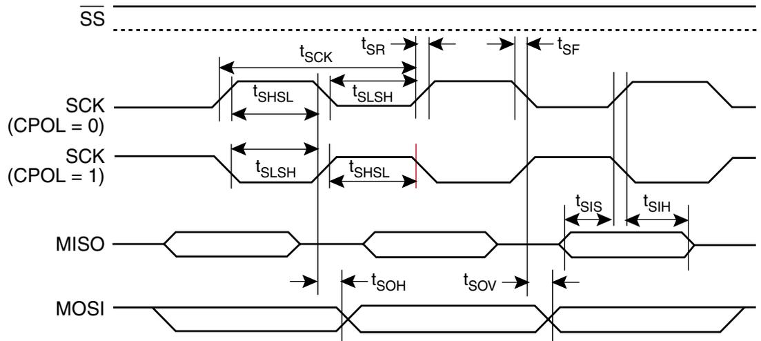
**Figure 15-5. SPI Slave Timing (CPHA = 0)**
