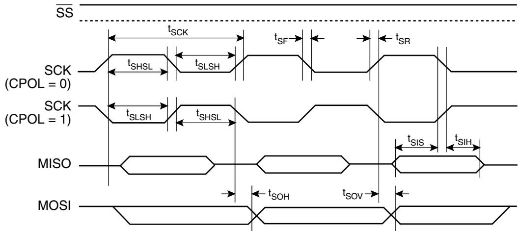
**Figure 15-7. SPI Slave Timing (CPHA = 1)**
