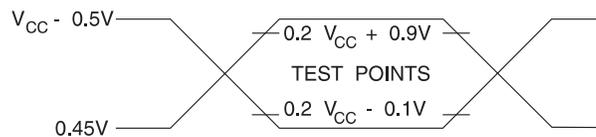
Note: 1. AC Inputs during testing are driven at  $V_{CC} - 0.5V$  for a logic 1 and  $0.45V$  for a logic 0. Timing measurements are made at  $V_{IH}$  min. for a logic 1 and  $V_{IL}$  max. for a logic 0.
