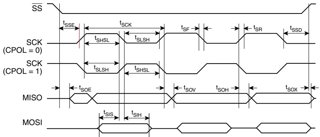
**Figure 15-8.** SPI Transfer Format with CPHA = 0
