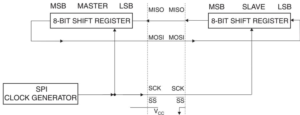
**Figure 15-2.** SPI Block Diagram
