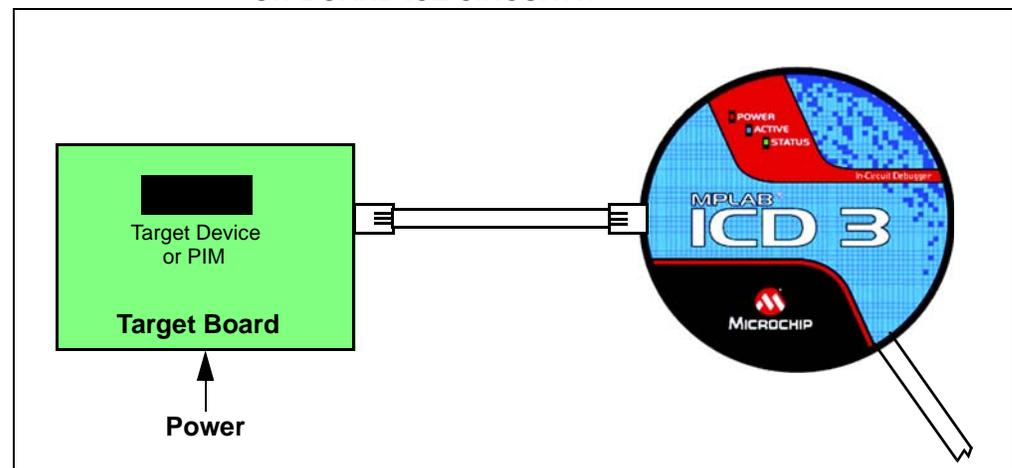
FIGURE 2-2: STANDARD DEBUGGER SYSTEM – ICE DEVICE
