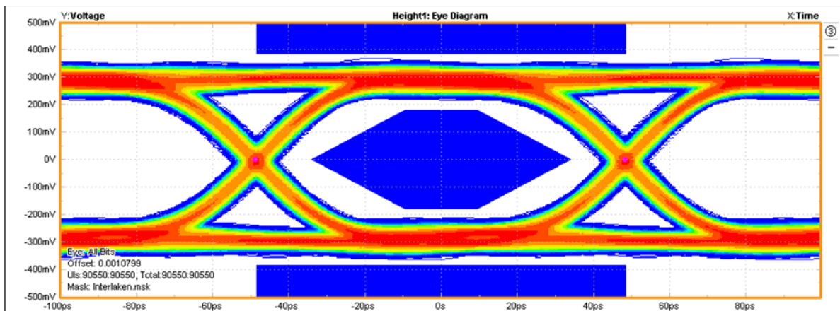
Figure 26 • Interlaken Data Eye Diagram
