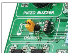
Figure 10-1: DS1820 connector (DS1820 is not connected)
