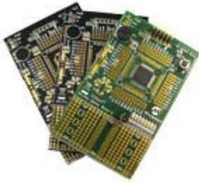
This is a small demo board with a PIC18F45K20 device on board and a small, surface-mount prototype area. Use it with a PICkit 3 In-Circuit Debugger to program your code via a 6-pin ICSP header on the board. This product also includes two bare PCB boards for those interested in customizing their development. This 44-Pin Demo Board also comes bundled with the PICkit 3 Debug Express if you order the DV164131.
