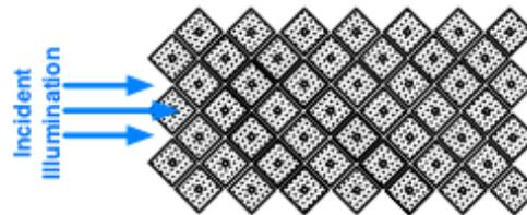
**Figure 1-4. 0.45-Inch DMD Diamond Pixel Array Configuration**
