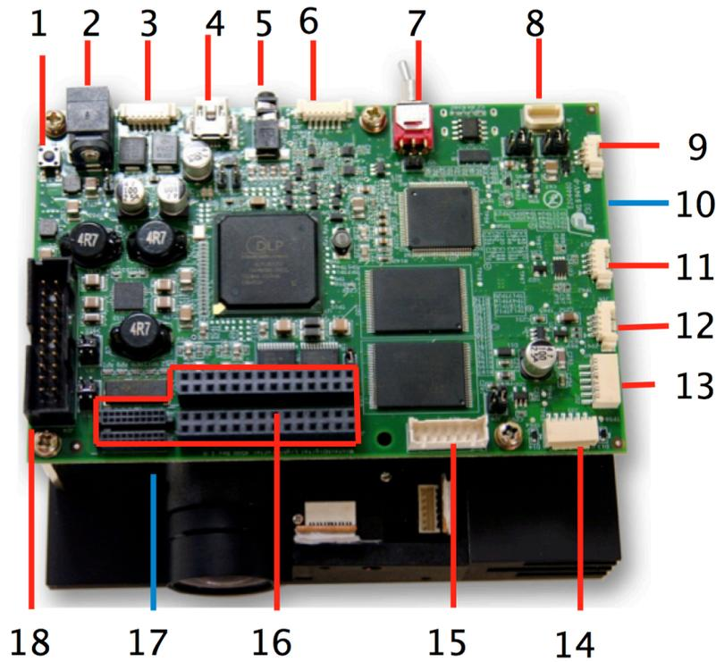
Figure 1-7. DLP LightCrafter 4500 Connectors (Top View)
