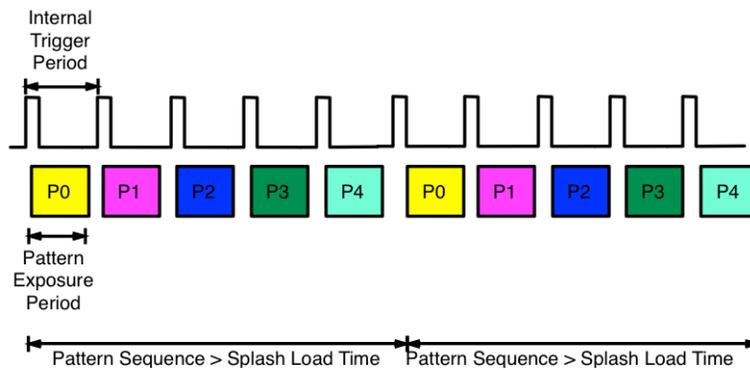
**Figure 4-5. Image Load Time and Pattern Sequence Timing**
