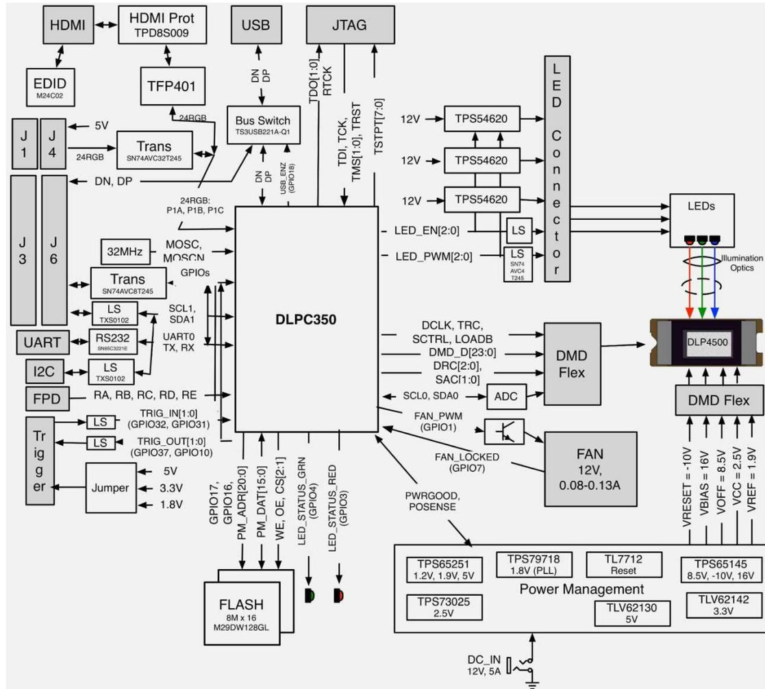
**Figure 1-6. DLP LightCrafter 4500 Driver Board Block Diagram**
