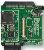
The Graphics LCD Controller PICTail Plus SSD1926 Board is a demonstration board for evaluating Microchip Technology's graphic display solution and graphics library for 16- and 32-bit microcontrollers. It is an expansion board compatible with the Explorer 16 development board (DM240001) or one of the PIC32 Starter Boards (DM320001,
