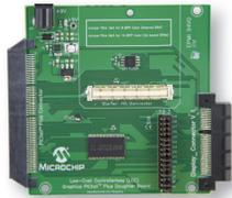
The Low-Cost Controllerless (LCC) Graphics PICTail Plus Daughter Board enables development of graphics solutions without an external graphics controller, thus reducing system BOM cost for many applications. The board is designed to attach to a PIC32 starter
