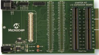
The PIC32 I/O Expansion Board provides Starter Kit and Starter Board users with full access to MCU signals, additional debug headers, and connection of PICTail Plus daughter
