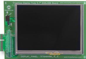
The Graphics Display Truly 5.7" 640 × 480 Board is a demonstration board for evaluating Microchip graphic display solution and graphics library for 16- and 32-bit microcontrollers.
