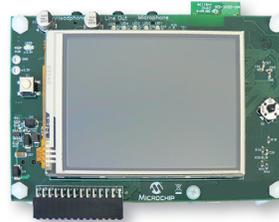
The Multimedia Expansion Board (MEB) provides PIC32 Starter Kit, dsPIC33E USB Starter Kit or PIC24E USB Starter Kit users with an integrated yet flexible solution for development of high impact user interfaces. The board comes with a 3.2" Color TFT touch-screen QVGA display, an onboard
