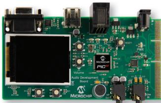
The audio Development Board for PIC32 MCUs features an 80 MIPS PIC32 MCU, a 24-bit Wolfson audio codec, a two-inch color LCD Display, a USB interface, and an onboard microphone. Supported by Microchip's
