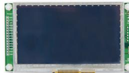
The PIC32 GUI development board with Projected Capacitive Touch enables development of cost effective multitouch graphical user interfaces. It provides USB host and device connectivity and
