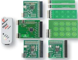
The enhanced mTouch Capacitive Evaluation Kit provides a simple platform for developing a variety of capacitive touch sense applications using PIC16F, PIC24F, PIC18F and PIC32 microcontrollers.
