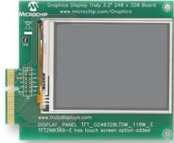
The Graphics Display Truly 3.2" 240 × 320 Board is a demonstration board for evaluating Microchip's graphic display solution and graphics library for 16- and 32-bit microcontrollers.
