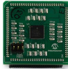
The PIC32MX250F128D PIM is designed to demonstrate the capabilities of the PIC32MX1XX/2XX family of devices using Explorer 16 Development Board. It enables USB and graphics development with the PIC32MX2XX series.
