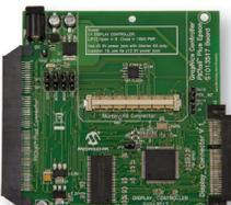
The Graphics Controller PICTail Plus Epson S1D13517 Board allows evaluating Microchip Technology's solution and graphics library for 16- and 32-bit microcontrollers. The Epson S1D13517 offers hardware acceleration for alpha-blending, transparency, animation,
