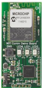
The PIC32 Wi-Fi Comm Demo board provides a compact development platform for customers to evaluate Microchip's Wi-Fi product offering. The demo board comes with onboard MRF24WB0MA Wi-Fi module which is FCC/IC/ETSI certified along with a PIC32 microcontroller.
