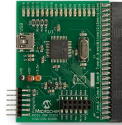
The PIC32 CTMU Evaluation Board is designed to facilitate the development of capacitive touch-based applications using the low cost high performance PIC32 MX1/MX2 -series microcontrollers. This evaluation board includes an on-board PICKit serial interface, an ICSP header, a USB connector (for power only), and 16 LEDs.
