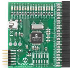
The PIC32 mTouch Capacitive Touch Evaluation Board is designed to facilitate the development of capacitive touch-based applications using PIC32-series microcontrollers. This evaluation board includes an on-board PICKit serial interface, an ICSP header, a USB connector
