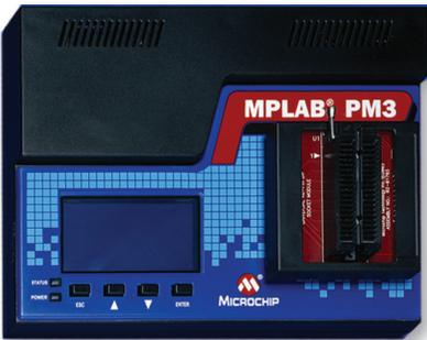
The MPLAB PM3 Universal Device Programmer is easy to use and operates with a PC or as a stand-alone unit. This development tool programs Microchip's entire line of PIC MCUs as well as the latest dsPIC DSC devices. When used
