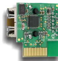
The Ethernet PICtail Plus Daughter Board provides a cost-effective method of evaluating and developing Ethernet control applications. The board is designed for flexibility and can be plugged into Microchip's Explorer 16 (DM240001) development board.
