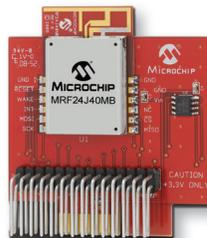
The MRF24J40MB PICtail/PICtail Plus Daughter Board is a demonstration and development daughter board for the MRF24J40MB 2.4 GHz IEEE Std. 802.15.4 20 dBm RF Transceiver Module. The daughter board can plug into multiple Microchip Technology Demonstration and development boards such as PIC18 Explorer
