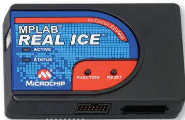
MPLAB REAL ICE In-Circuit Emulator System is Microchip's high-speed emulator for Microchip Flash DSC and MCU devices. It debugs and programs PIC microcontrollers and dsPIC DSCs with the easy-to-use
