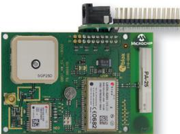
Microchip's Machine-to-Machine (M2M) PICtail Daughter Board (AC320011) based upon u-blox GPS and GSM/GPRS modules makes it easy to create low-cost M2M applications with location-awareness capabilities. The daughter board can be interfaced
