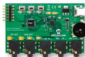
The PIC32 USB Digital Audio Accessory Board showcases a 16/24-bit quality digital stereo audio development platform using the PIC32 microcontroller (MCU). It can be used for 16/24-bit stereo audio playback and recording
