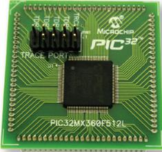
This Plug-In Module enables PIC32 development on the Explorer 16 Development Board (DM24000X) and supports the MPLAB REAL ICE In-Circuit Emulator Trace Kit (AC244006). An 80 MHz PIC32MX360F512L with 512 KB of Flash, 32 KB of RAM, 4 channels of hardware DMA, and instruction trace is installed on the plug-in module.
