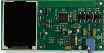
The PIC32 MX1/ MX2 Starter kit (DM320013) is a complete solution for exploring the low-cost, high-performance PIC32MX1/MX2 devices. This kit is perfect for
