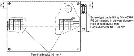
Tightening torque 1.5 ... 1.8 Nm
