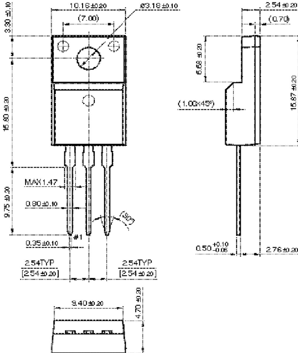
\* Front/Back Side Isolation Voltage : AC2500V
