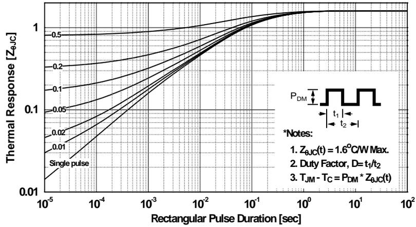
Figure 13. Transient Thermal Response Curve-FDPF5N50NZ
