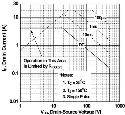
Figure 10. Maximum Safe Operating Area vs. Case Temperature-FDPF5N50NZ
