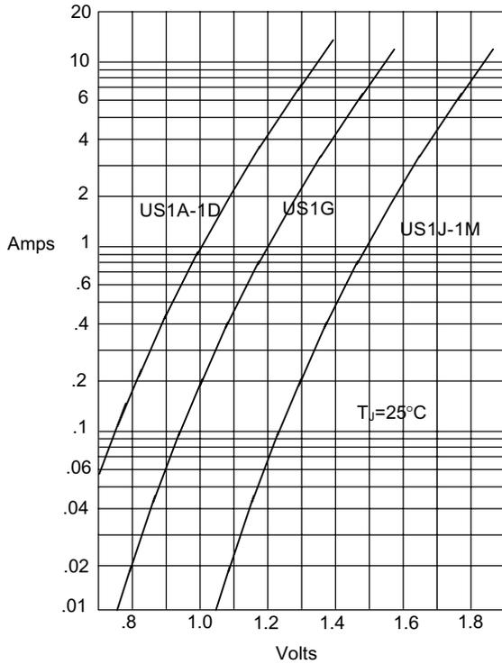
Instantaneous Forward Current - Amperes versus
