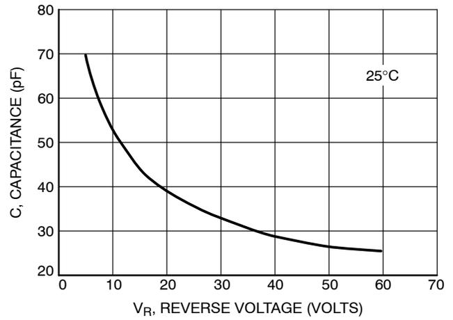
Figure 4. Typical Capacitance
