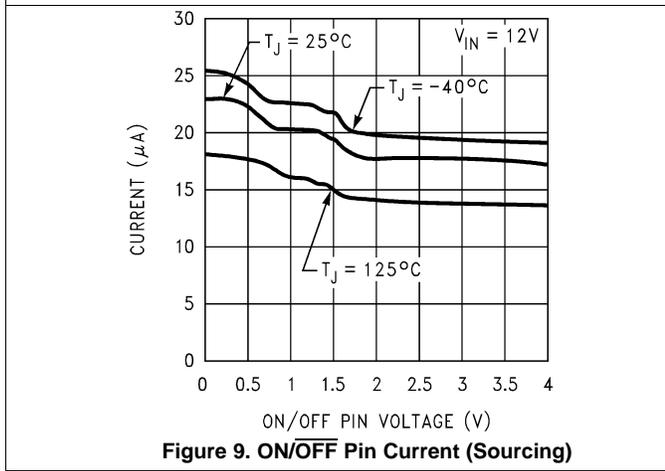
Figure 9. ON/OFF Pin Current (Sourcing)
