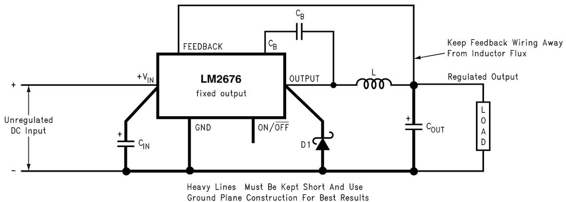
Figure 21. Basic Circuit for Fixed Output Voltage Applications.
