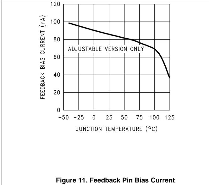
Figure 11. Feedback Pin Bias Current
