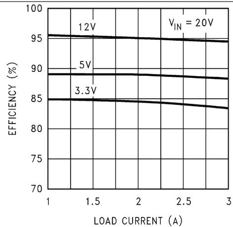
Figure 4. Efficiency versus I<sub>LOAD</sub>
