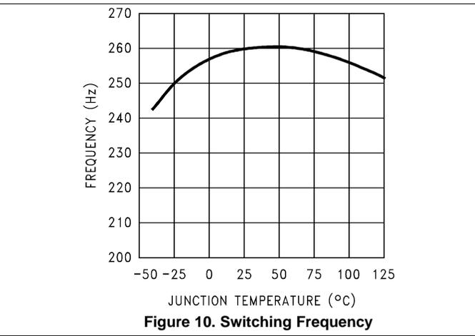
Figure 10. Switching Frequency
