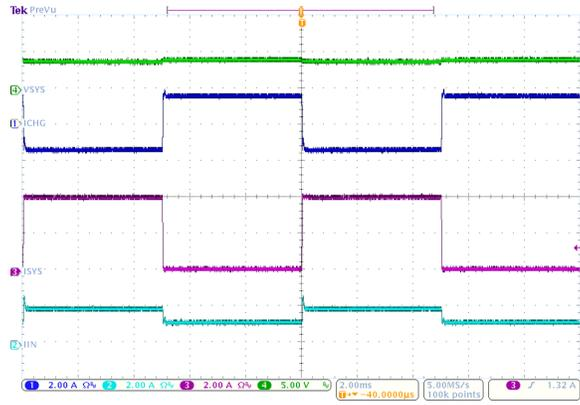
$I_{SYS} = 0 - 4 \text{ A}$        $V_{VBUS} = 5 \text{ V}$        $I_{INDPM} = 2 \text{ A}$
