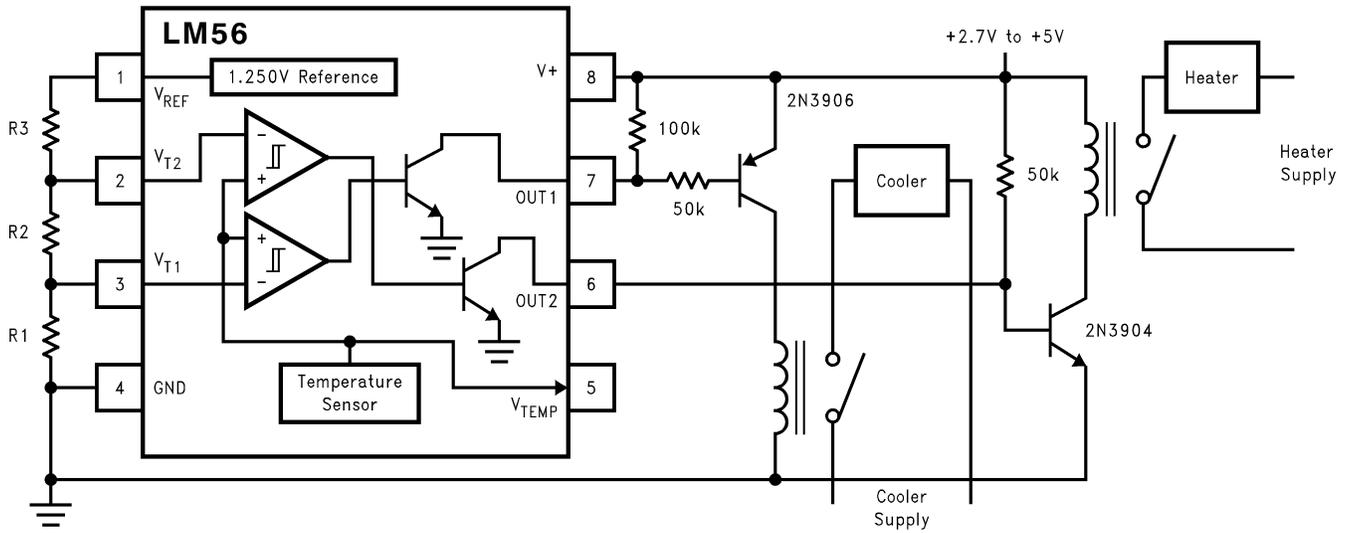
Figure 19. Simple Thermostat
