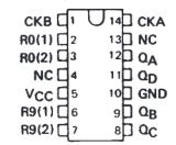
SN5492A, SN54LS92...J OR W PACKAGE SN7492A...N PACKAGE SN74LS92...D OR N PACKAGE (TOP VIEW)
