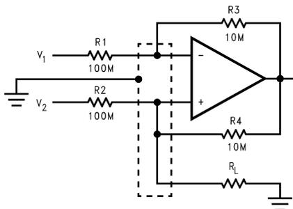
Figure 23. Guard Ring Connections: Howland Current Pump
