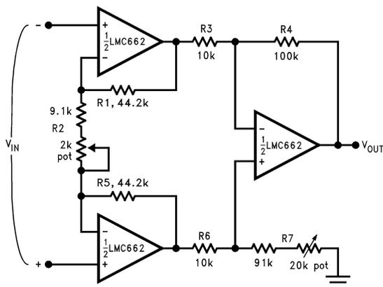
If  $R_1 = R_5$ ,  $R_3 = R_6$ , and  $R_4 = R_7$ ; then
