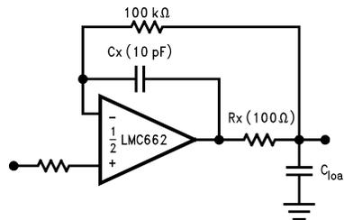
Figure 17. Rx, Cx Improve Capacitive Load Tolerance
