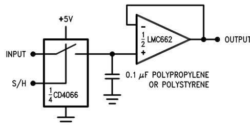
**Figure 26. Low-Leakage Sample-and-Hold**
