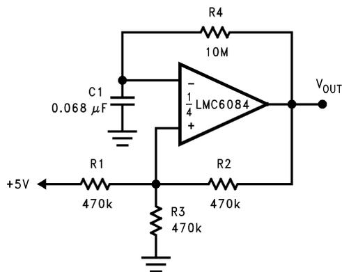
**Figure 33. 1 Hz Square Wave Oscillator**
