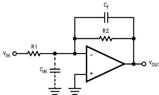
Figure 25. Cancelling the Effect of Input Capacitance
